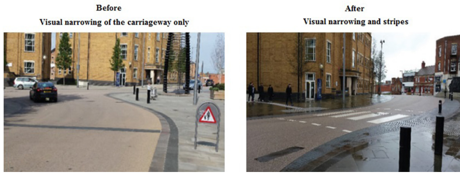
Fig. 3. Kimbrose Triangle: before and after, Source: CIHT (2018) Creating better streets: Inclusive and accessible places. CIHT, London., p.97. Reproduced with written permission from the publisher.
